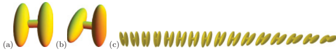
FIG. 1. (Color online) (a) Achiral and (b) chiral biaxial molecular structures studied in this work. (c) Cholesteric phase of chiral molecules, showing the macroscopic twist.
