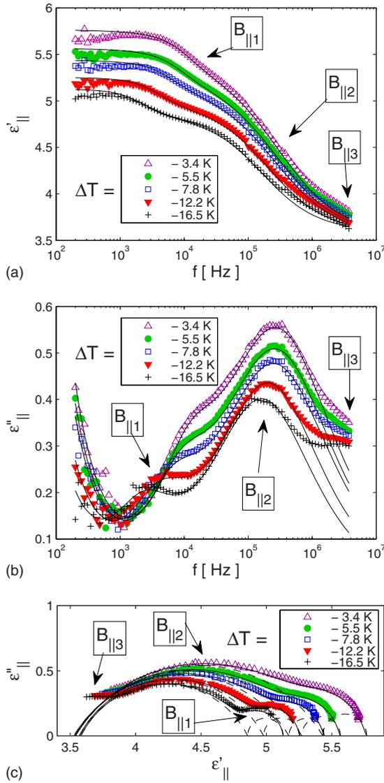
FIG. 3. (Color online) Frequency dependence of the parallel component of the (a) permittivity  $\epsilon'_{||}$  and the (b) loss  $\epsilon''_{||}$  in the nematic phase of CIPbis10BB at various  $\Delta T = T - T_{NI}$  temperatures. (c) The corresponding Cole-Cole plot. Symbols are measured values, solid lines correspond to a fit with two relaxations. The dashed lines show the two fitted relaxations separately.
