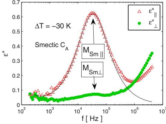
FIG. 11. (Color online) Frequency dependence of the perpendicular and the parallel components of the loss in the  $\text{SmC}_A$  phase of the mixture with  $X=0.5$  at 30 K below  $T_{Nf}$ . Symbols are measured values, the solid line corresponds to a fit with one dispersion.
