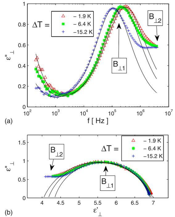
FIG. 4. (Color online) (a) Frequency dependence of the loss  $\epsilon''_{\perp}$  for the perpendicular component in the nematic phase of CIPbis10BB at various  $\Delta T = T - T_{NI}$  temperatures. (b) The corresponding Cole-Cole plot. Symbols are measured values, solid lines correspond to a fit with one relaxation.
