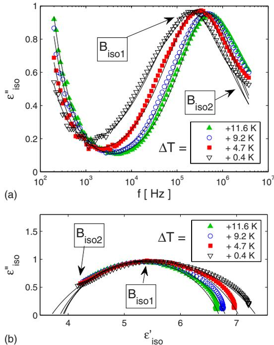
FIG. 6. (Color online) (a) Frequency dependence of the loss  $\epsilon''_{iso}$  in the isotropic phase of CIPbis10BB at various  $\Delta T = T - T_{NI}$  temperatures. (b) The corresponding Cole-Cole plot. Symbols are measured values, solid lines correspond to a fit with one relaxation.
