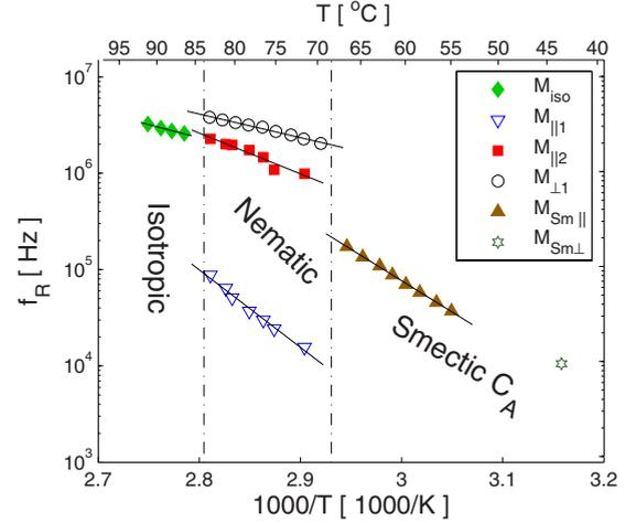
FIG. 12. (Color online) Temperature dependence of the relaxation frequencies in the isotropic, nematic, and smectic phases of the mixture with  $X=0.5$  molar fraction of 6OO8 in CIPbis10BB. Symbols are measured values, solid lines correspond to a fit to Eq. (2).
