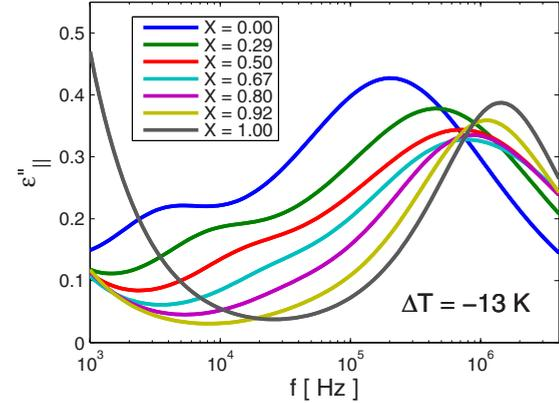
FIG. 13. (Color online) Synthesized dielectric spectrum of the parallel component of the loss for binary mixtures of ClPbis10BB/6O08 assuming three dispersions.
