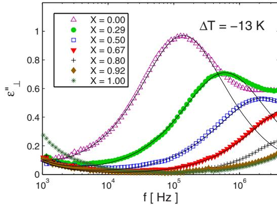
FIG. 9. (Color online) Frequency dependence of the perpendicular component of the loss  $\varepsilon''_{\perp}$  in the nematic phase of binary mixtures of CIPbis10BB/6OO8 at various concentrations of the calamitic compound at the relative temperature  $\Delta T = -13$  K. Symbols are measured values, solid lines correspond to a fit with one relaxation.
