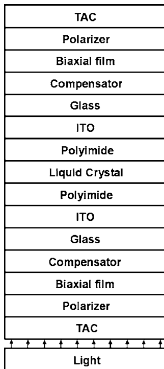
FIG. 8. Optical stack of the real pi cell. All layers are combined as a single unit without any air gaps.
