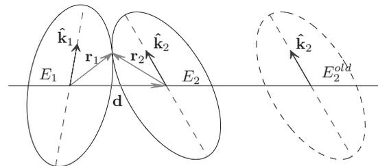
FIG. 1. Two externally tangent ellipses  $E_1$  and  $E_2$ . The directions of the major axes are given by  $\hat{\mathbf{k}}_1$  and  $\hat{\mathbf{k}}_2$ ; the centers are joined by the vector  $\mathbf{d}$ .
