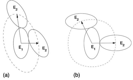
FIG. 3. Excluded area for two ellipses. Ellipse  $E_1$  is fixed at the origin, and ellipse  $E_2$  rotates around it, keeping its orientation fixed and remaining tangent to  $E_1$ . The center of  $E_2$  traces out the dashed curve. The area bounded by the dashed curve is the excluded area  $A_{ex}$ .
