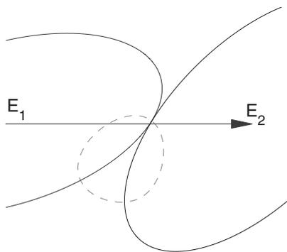
FIG. 4. Locus of the point of contact. Ellipse  $E_1$  is rotated about its center, while ellipse  $E_2$  keeps its orientation fixed. The center of  $E_2$  moves so that  $E_2$  remains tangent to  $E_1$ . The point of contact traces out the dashed curve.
