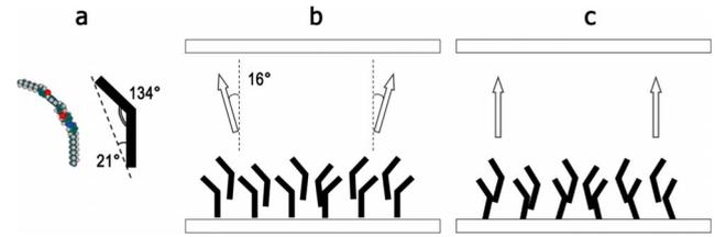
FIG. 4. (Color online) (a) Optimized structure of A131 by quantum-chemical calculations (MOPAC method, AM1 Hamiltonian) with a bend angle of  $134^\circ$ , which agrees quite well with the NMR result [16]. (b),(c) Schematic illustration of the orientation of bent-core molecules near the alignment layer's boundary and resulting tilting directors (arrows) of two adjacent domains in the bulk (b) without field and (c) with very high field.
