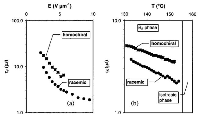
FIG. 5. Temperature (a) and electric field dependence (b) of the switching time,  $\tau_s$ , of a  $10 \mu\text{m}$  cell, as determined by the time needed to reach the maximum polarization current following field reversal.
