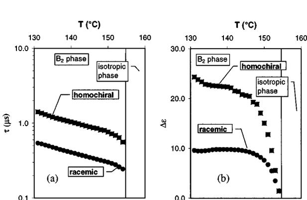
FIG. 3. (a) Temperature dependence of the relaxation time determined from the maximum of Fig. 2 as  $\tau=2\pi/f$ . (b) Temperature dependence of  $\Delta\epsilon$ .
