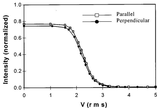
FIG. 5. Measured first five odd orders from ZLI-4792 filled Orthogonal-Twist grating, for first optimal  $\Delta nd/\lambda$  value. Electro-optical response measured for incident polarizations parallel and perpendicular to the grating stripes.
