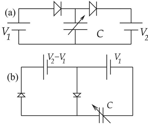
FIG. 1. (a) Charge pump: model circuit. Charge is pumped from the source  $V_1$  to the higher voltage  $V_2$ . (b) A more practical circuit which recharges the source battery.
