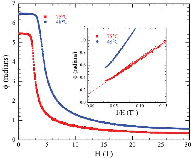
FIG. 3. (Color online) Optical phase difference (for a 5.5  $\mu\text{m}$  thick sample and  $\lambda = 632.8$  nm) vs magnetic field at two different temperatures. The Freedericksz transition is clearly seen below 5 T. Inset: Behavior at very large fields. In both cases the phase difference at infinite field is positive.
