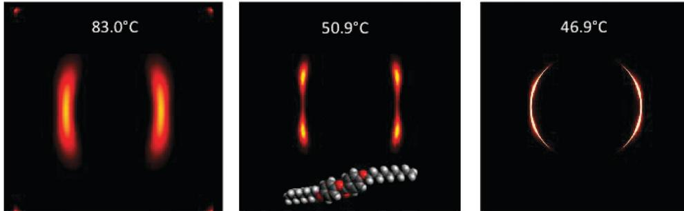
FIG. 1. (Color online) SAXS diffraction intensities at three different temperatures. The x-ray wavelength employed was  $0.775 \text{ \AA}$  and there is a  $\sim 1 \text{ T}$  magnetic field applied horizontally. The centers of the diffuse peaks in the middle image lie at  $q = 0.23 \text{ \AA}^{-1}$  and at an angle  $31^\circ$  to the horizontal which corresponds to a layer periodicity of  $27.3 \text{ nm}$ . The molecular structure of 6OO8 is shown in the inset.
