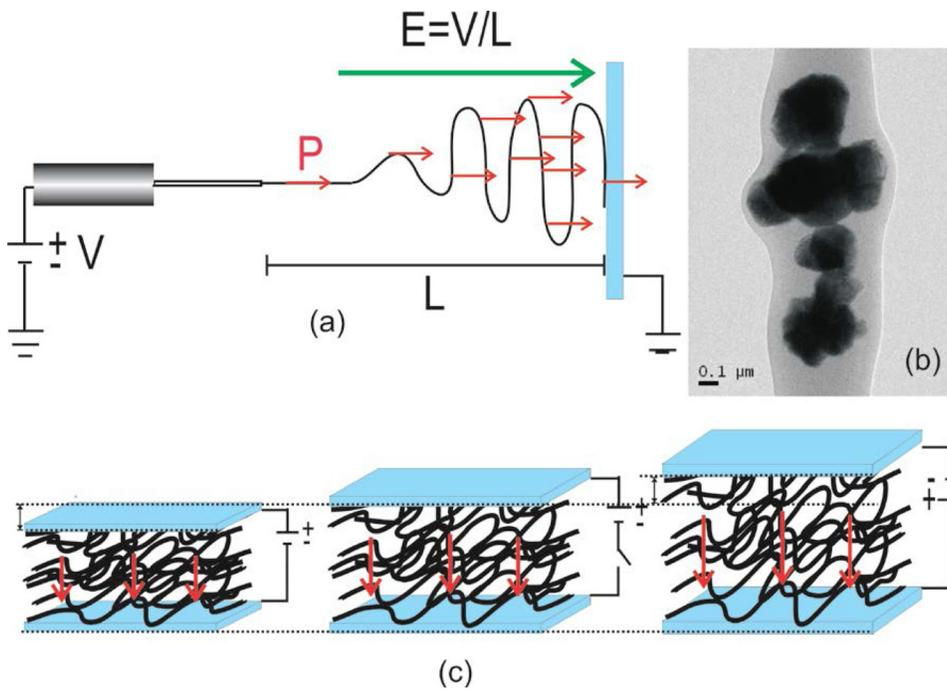
FIG. 1. (Color online) Illustration of the experimental procedures, fiber structure, and the physical model of piezoelectric response of the PLA/BT fiber mat: (a) Sketch of the standard electro-spinning process and poling; (b) TEM nanostructure of a fiber including BT particles (dark areas); and (c) sketch of the piezoelectric response when the external field is parallel, zero, and anti-parallel with the polarization of the BT nanoparticles, from left to right.
