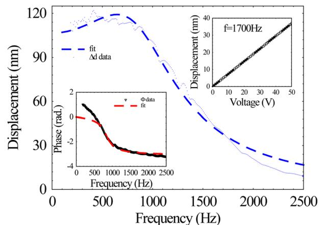
FIG. 3. (Color online) Frequency dependence of the displacement of the cover glass plate of  $m_g = 2.5 \text{ g}$  measured by a  $m_a = 2.5 \text{ g}$  accelerometer at  $50 \text{ V}$  applied, and of the fit of a forced damped oscillator (dotted line). Right upper inset: the voltage dependence of the displacement at  $1700 \text{ Hz}$ . Left lower inset: The frequency dependence of the phase in radians and a fit (dotted line).
