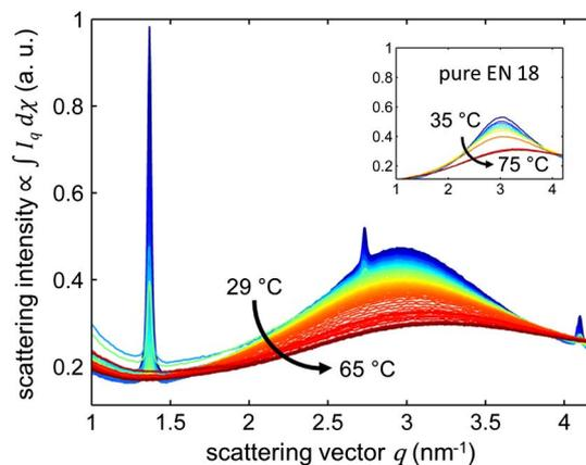
Fig. 3. (Color online) Scattering intensity versus magnitude of the scattering vector recorded for a capillary filled with BaTiO<sub>3</sub>-nanoparticle-doped EN18. The sample was slowly heated from 29°C (blue curves) to 65°C (red curves). The inset shows scattering curves observed for the pure LC.
