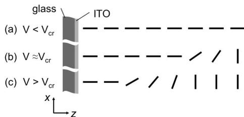
Fig. 4. Fredericks transition in an LC test cell with homeotropic anchoring: schematic plots of the director field near one glass boundary (a) if no voltage is applied (b), if a voltage near the critical voltage is applied, and (c) if a voltage larger than the threshold voltage is applied.
