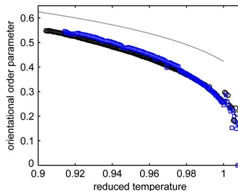
Fig. 2. (Color online) Orientational order parameter versus reduced temperature, as calculated by the Maier-Saupe theory (solid line), observed upon heating pure EN18 (circles) and doped EN18 (squares).
