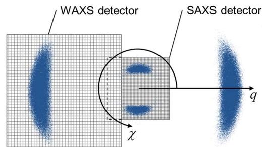
Fig. 1. (Color online) Scheme of the oriented 2D diffraction pattern of a nematic LC, a coordinate system based on the angle  $\chi$  and the scattering vector  $q$ , and the alignment of two detectors, which cover the SAXS and the WAXS angular regions, respectively.
