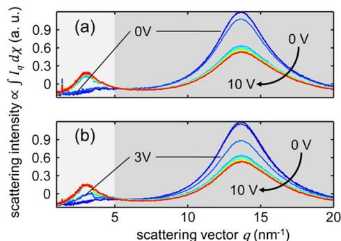
Fig. 5. (Color online) Scattering intensity versus magnitude of the scattering vector recorded for planar LC test cells. The addressing voltage is varied from 0 (blue curves) to 10 V (red curves) in steps of 1 V. (a) Pure EN18. (b) EN18 doped with harvested  $\text{BaTiO}_3$  nanoparticles.
