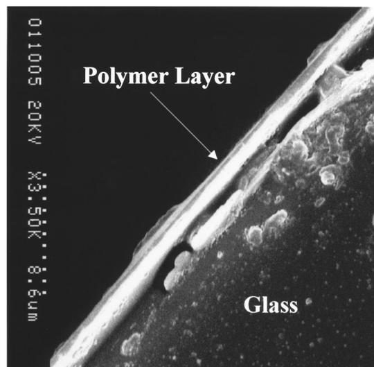
FIG. 3. SEM image showing substrate and polymer film.
