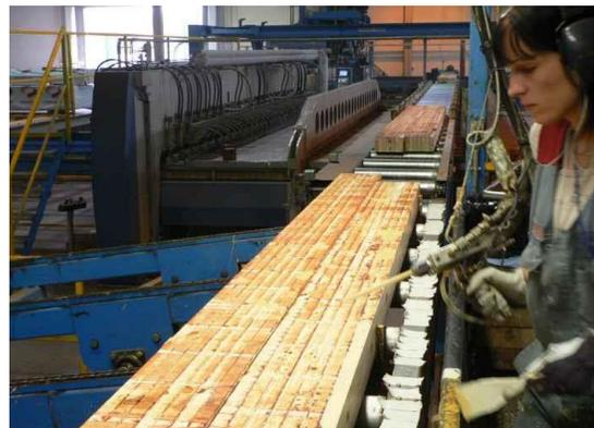
Above is depicted a woman applying sealant to a beam that has already been assembled. Note how the beam is just a composition of layers of dimension lumber. (source: gate-project.org)
