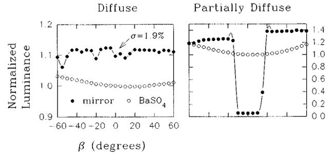
FIG. 2. Luminance as a function of the viewing angle ( $\beta$ ) for a mirror and a white standard, BaSO<sub>4</sub>, using diffuse and partially diffuse illumination. The term  $\sigma$  denotes the standard deviation indicating the diffuse source is diffuse within  $\sim 1.9\%$ . The horizontal axes are scaled the same.
