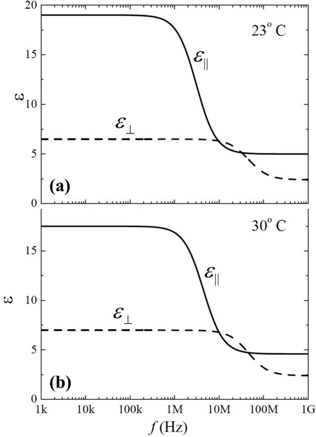
FIG. 2. Dielectric dispersion curves of 5CB based on the Debye model, Eq. (24), where  $\epsilon_{||}=19.0$ ,  $\epsilon_{h||}=5.0$ , and  $\tau_{||}=64$  ns;  $\epsilon_{l\perp}=6.5$ ,  $\epsilon_{h\perp}=2.4$ , and  $\tau_{\perp}=3.5$  ns for 23 °C (a) and  $\epsilon_{||}=17.5$ ,  $\epsilon_{h||}=4.6$ , and  $\tau_{||}=36$  ns;  $\epsilon_{l\perp}=7$ ,  $\epsilon_{h\perp}=2.4$ , and  $\tau_{\perp}=3.5$  ns for 30 °C (b).
