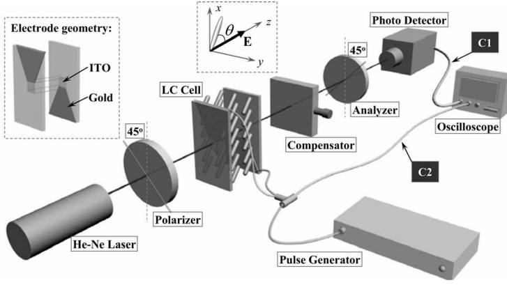
FIG. 1. Experimental setup for the DME experiment.
