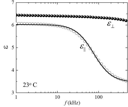
FIG. 7. Dielectric dispersion curves for the real components ( $\varepsilon_{\parallel}$ ,  $\varepsilon_{\perp}$ ) of the mixture 53.7 wt. % MLC7026-100+46.3 wt. % MLC2048 at 23 °C. The solid curve is fitted with Eq. (24) where  $\varepsilon_{f\parallel} = 3.5$ ,  $\varepsilon_{f\parallel} = 6.0$ , and  $\tau_{\parallel} = 2.1 \mu\text{s}$ .
