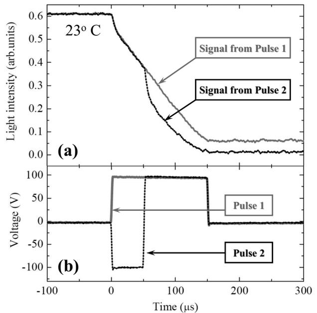
FIG. 10. Transmitted light intensity versus time (a) for the cell filled with the mixture 53.7 wt. % MLC7026-100+46.3 wt. % MLC2048, driven by a dc pulse 1 of duration of  $150\ \mu\text{s}$  and amplitude 100 V and by a pulse 2 with a total duration  $150\ \mu\text{s}$  and amplitude  $\pm 100\ \text{V}$ , with polarity changed once (b).
