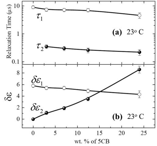
FIG. 5. The first and second dielectric relaxation times (a) and dielectric strength (b) of the parallel component  $\epsilon_{\parallel}$  of 5CB +MLC2048 mixtures versus the weight concentration of 5CB at 23 °C.
