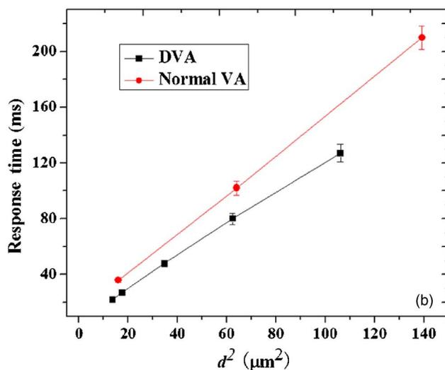
FIG. 2. (a) Response time of the DVA cells as a function of  $d/p$ ; (b) response time vs  $d^2$  for unrubbed VA cells with  $d/p=0$  and for DVA cells with  $d/p \approx 0.23$ . The measurements were performed using a He-Ne laser light with the wavelength  $\lambda=633 \text{ nm}$ .
