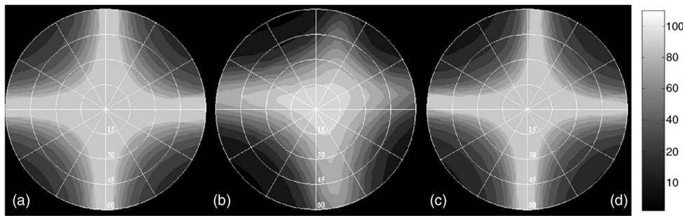
FIG. 4. Iso-contrast plots for viewing angle performance of (a) a normal PVA cell ( $d/p=0, d \approx 4 \mu\text{m}$ ), (b) a DVA cell ( $d/p \approx 0.23, d \approx 4 \mu\text{m}$ ), and (c) a PDVA cell ( $d/p \approx 0.23, d \approx 8 \mu\text{m}$ ); the relative intensity scale bar is shown in (d). The measurements were performed using white achromatic light.
