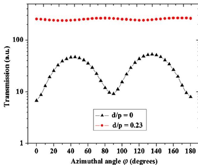
FIG. 3. Light transmission as a function of the azimuthal angle  $\phi$  for DVA cells with  $d/p=0$  and  $d/p \approx 0.23$  under  $U=6 \text{ Vrms}$  at 1 KHz. The measurements were performed using a monochromatic light with the wavelength  $\lambda=546 \text{ nm}$ .
