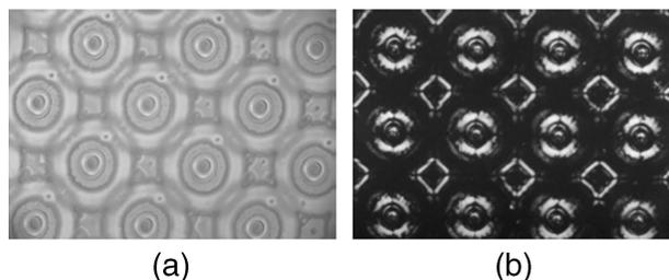
Fig. 2. Microscopic textures of a microlens array under a polarizing microscope with no voltage applied. The rubbing direction is rotated (a)  $45^\circ$  and (b)  $0^\circ$  with respect to one of the crossed polarizers. Concentric rings of different colors signify changing optical thicknesses, and areas of uniform shading outside the lenses indicate cell uniformity.
