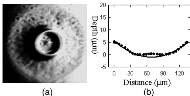
Fig. 5. (a) Microscopic structure and (b) depth profile of one of the microlenses. The curve in (b) is a fit to determine the radius of curvature,  $R = 381 \pm 20 \mu\text{m}$ , and the diameter,  $\sim 150 \mu\text{m}$ .
