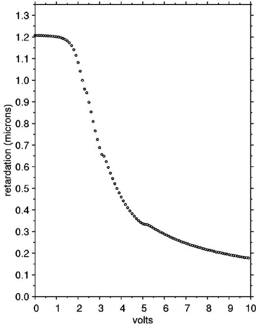
Fig. 2 Optical phase delay versus voltage for 6.0 μm cell.
