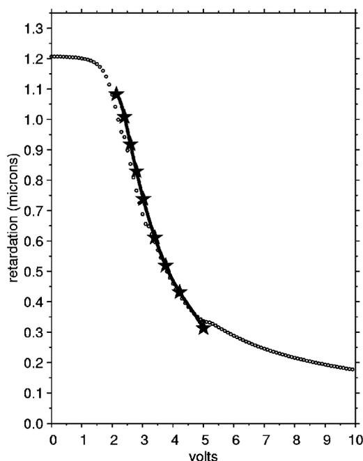
Fig. 5 Original optical phase delay with correcting spline.
