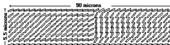
**Fig. 11** Conformation for a  $d=5.5 \mu\text{m}$  ideal cell.
