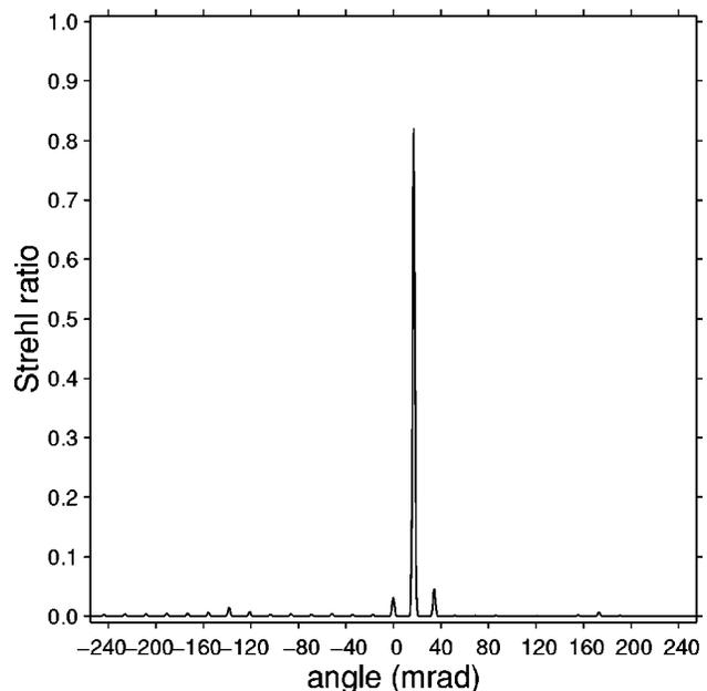
Fig. 7 Far-field diffraction pattern for device of Fig. 6.
