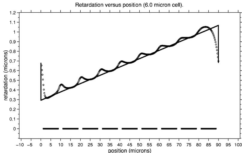
Fig. 6 Optical phase delay using revised voltages.
