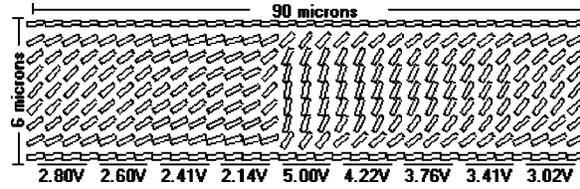
Fig. 3 Conformation (centered at the reset) for one blaze of a 6.0 μm cell.
