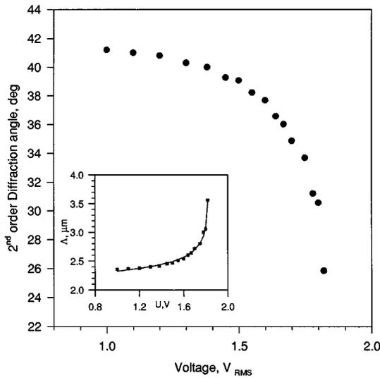
FIG. 3. Direction of the second diffraction maximum and the grating period  $\Lambda$  [calculated from Eq. (2)] as the function of the voltage applied to the cell No. 2. Experimental data  $\Lambda(U)$  are fitted by Eq. (3) with  $U_C = 1.85$  V ( $U_C = E_C \cdot d$ ) and equilibrium pitch  $p = 1.95 \mu\text{m}$ .
