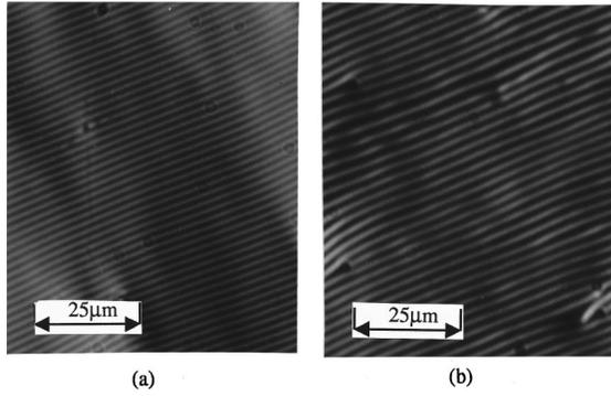
FIG. 2. Polarizing-microscope textures of the  $M$  state in cell No. 2 with modulations in the plane of the cell. The period of modulations changes with the applied voltage  $U$ : (a)  $U = 1.1$  V, (b)  $U = 1.75$  V.
